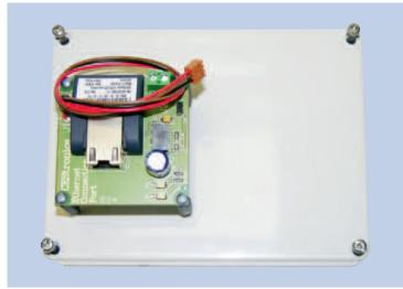
For existing installations, the CEMO control systems (type without integrated power supply unit) can be easily upgraded to a CEMO-NET online version.
